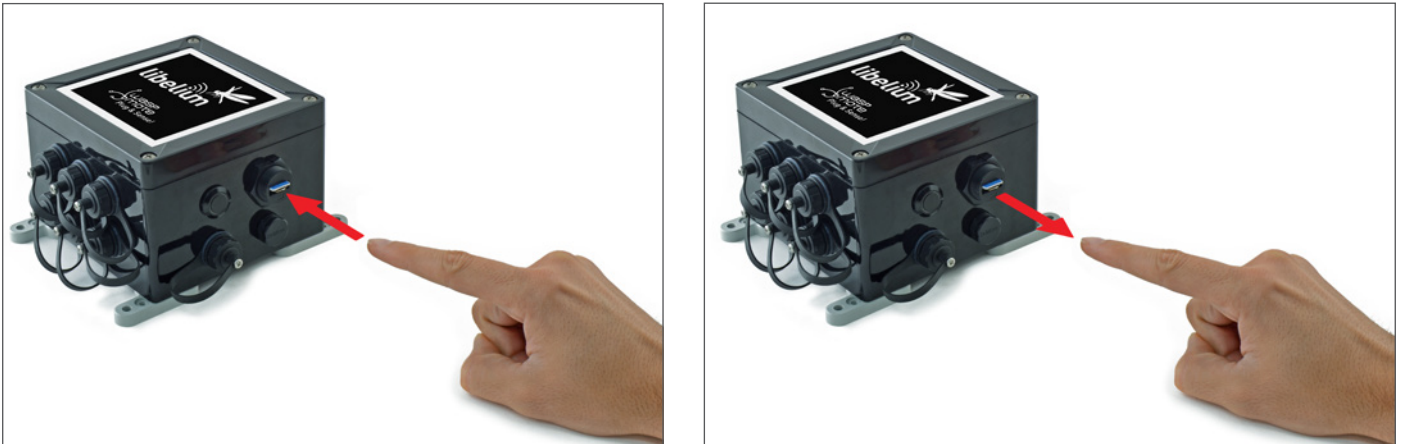
Figure: Push-pull mechanism in the External SIM socket
