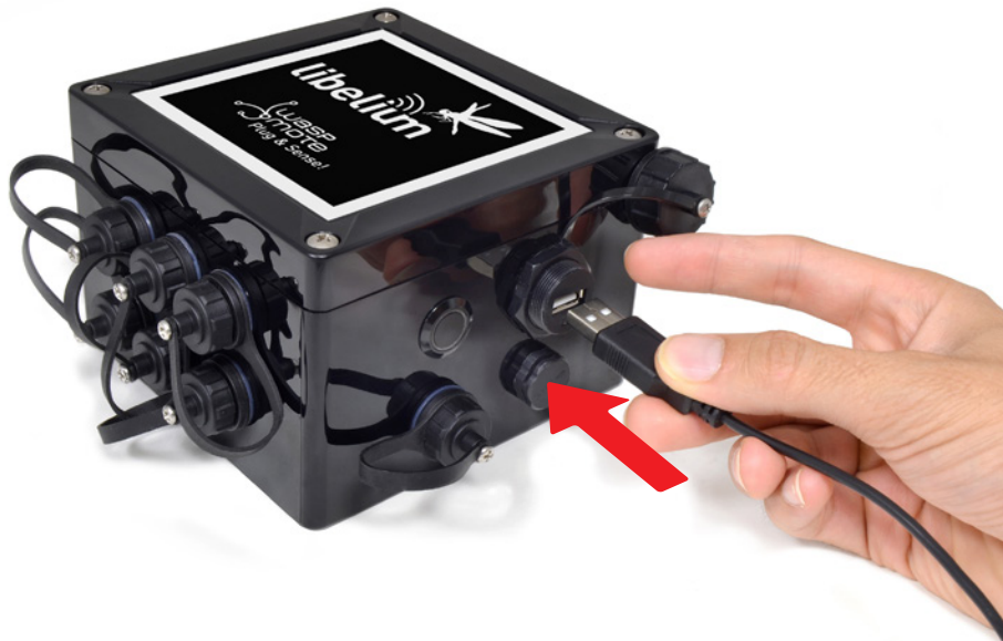
Figure: USB connector and protective cap
