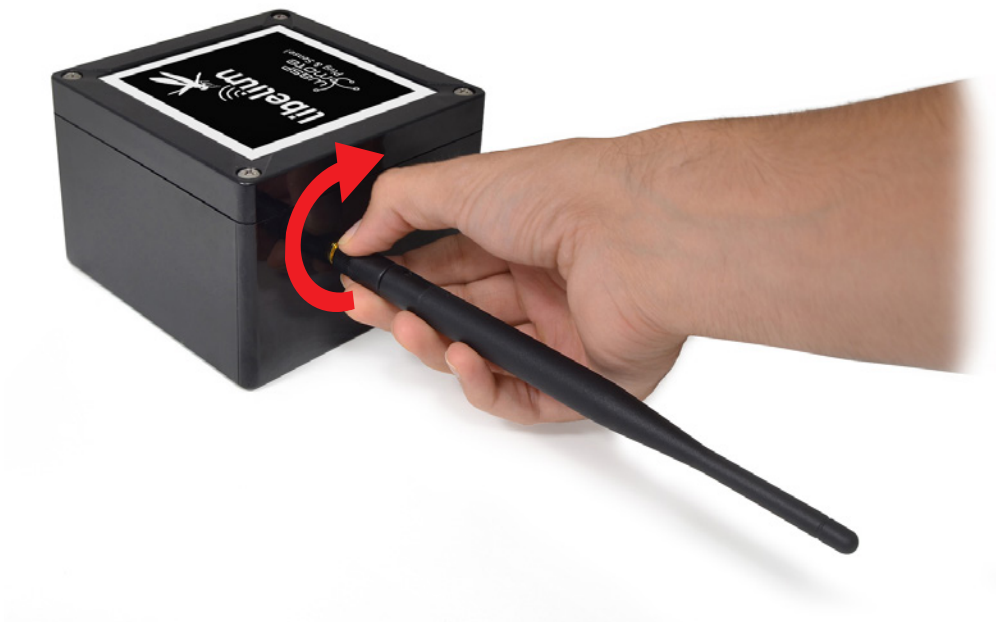
Figure: Connecting antenna to the enclosure
