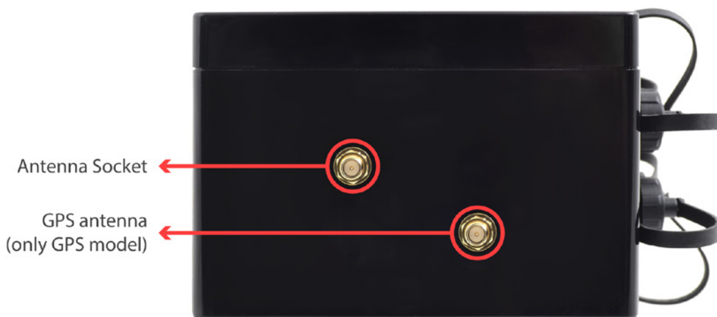
Figure: Main and GPS antennas connectors (only GPS-ready models)
