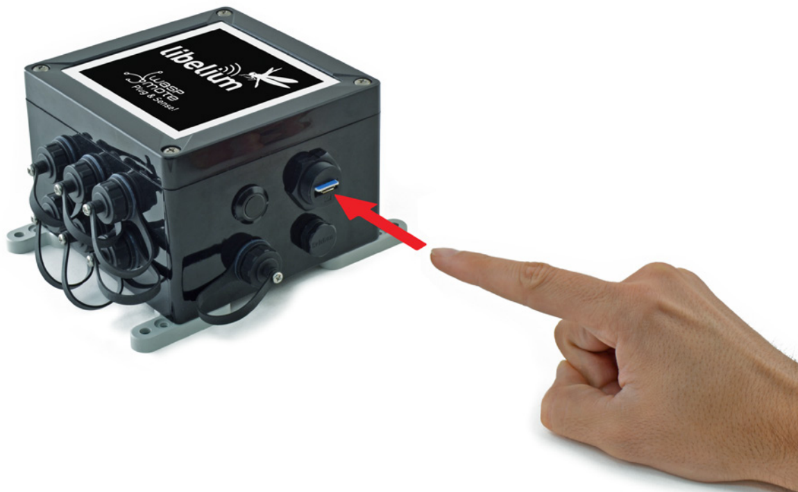
Figure: Inserting a SIM card with care in the External SIM socket
