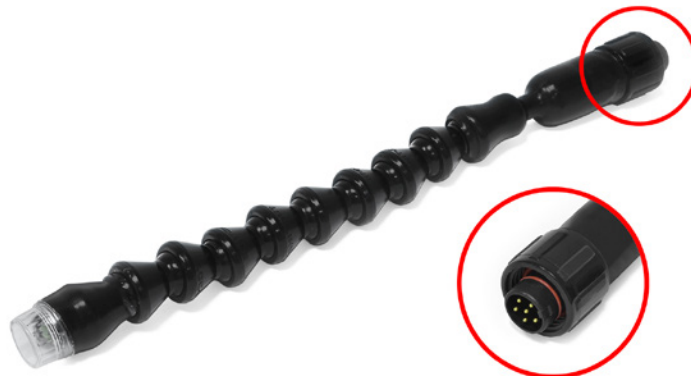
Figure: Luminosity (luxes accuracy) directionable probe
