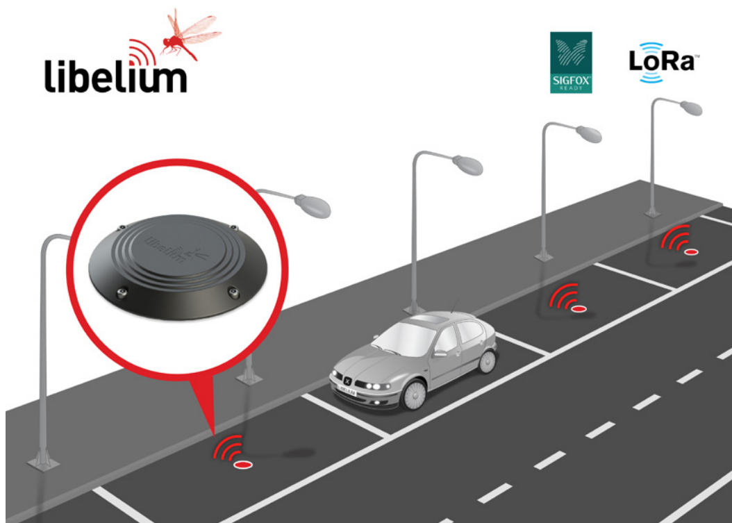
Figure: Smart Parking application diagram
