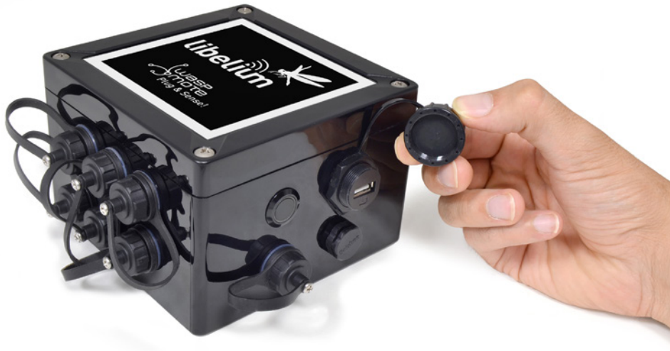
Figure: USB connector and protective cap
